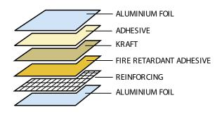
Antiblaze 760 is a medium weight 6 layer laminate with one non scuff Albar surface. A supporting mesh is required when installing Antiblaze 760 across spans greater than 600mm.
