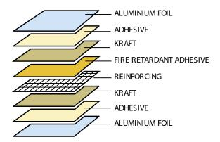
Antiblaze® 990 is a heavy weight 8 layer laminate consisting of two non scuff Albar faces. The exceptionally high tensile strength of Antiblaze® 990 allows installation aross spans of up to 1200mm without requiring a supporting mesh.
