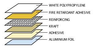
Antiblaze® Whitecap® is a medium weight 6 layer laminate consisting of one non scuff aluminium surface and one non scuff white polypropylene laminate.
